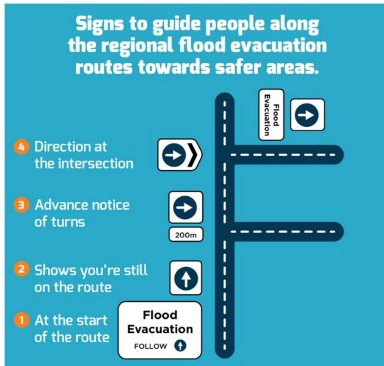
Representation of flood evacuation route signage installed in the Hawkesbury-Nepean Valley. Image: NSW SES
