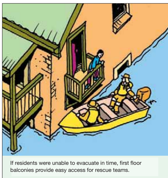
Figure 48 The advantage of balconies on two-storey houses
