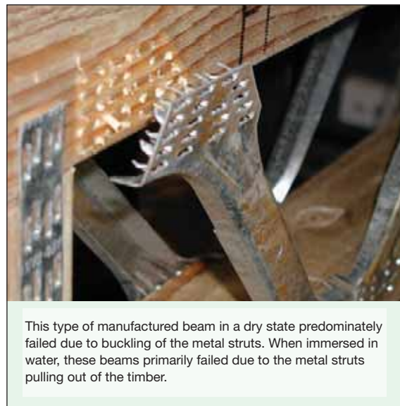
Figure 77 Beam failure
